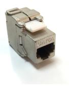
D-Link Category 6A FTP keystone jacks are RJ45 8P 8C 50u Jacks suitable for 22-24 AWG stranded and solid wire, toolless and compatible with both 110 & Krone punch down tools. They fit in high density keystone patch panel. Compliant with TIA/EIA 568A and B.
